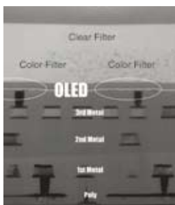
Multifunction LSI cross-section
