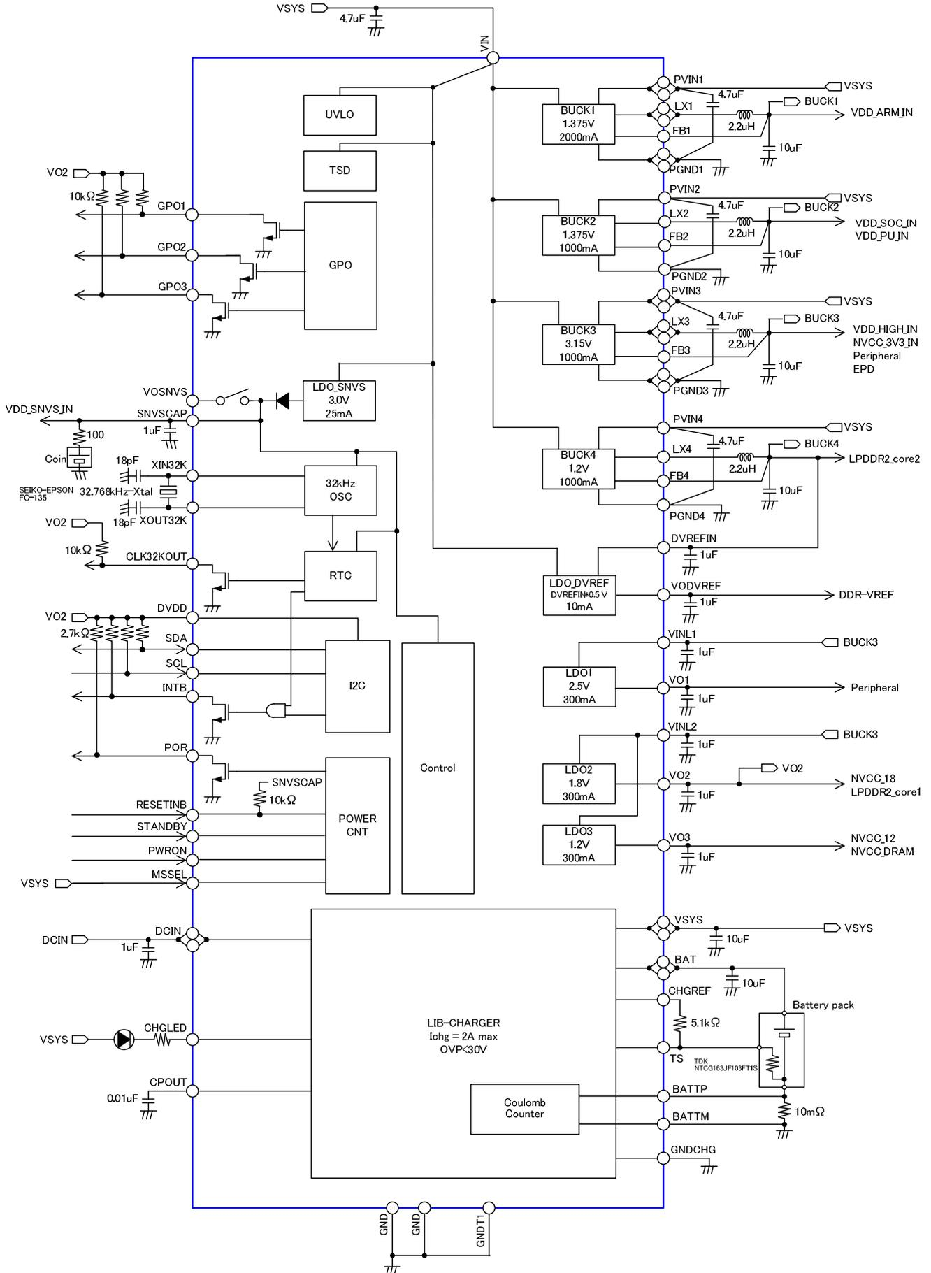
Figure 4. IC Block Diagram (Slave Control Mode)
