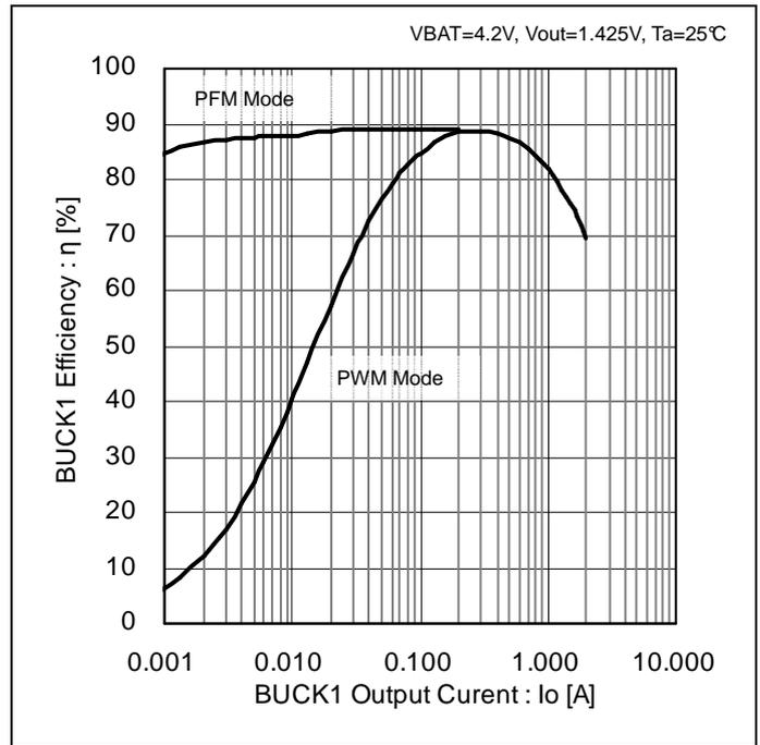
Figure 7. BUCK1 – Efficiency (PWM Mode / PFM Mode)
