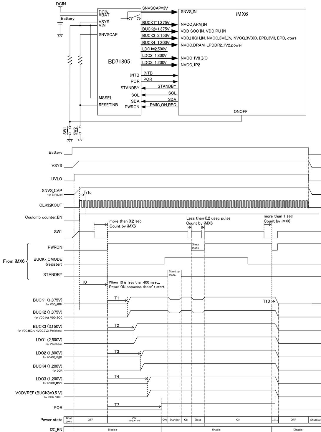
Figure 15. Power-ON/OFF Sequence (Slave control mode)
