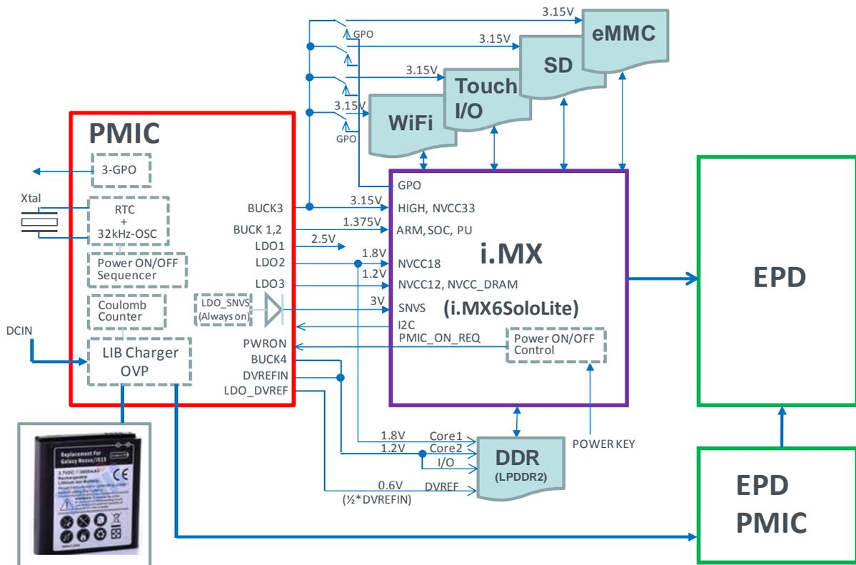
Figure 2. Typical Applications 2 (Slave Control Mode)
