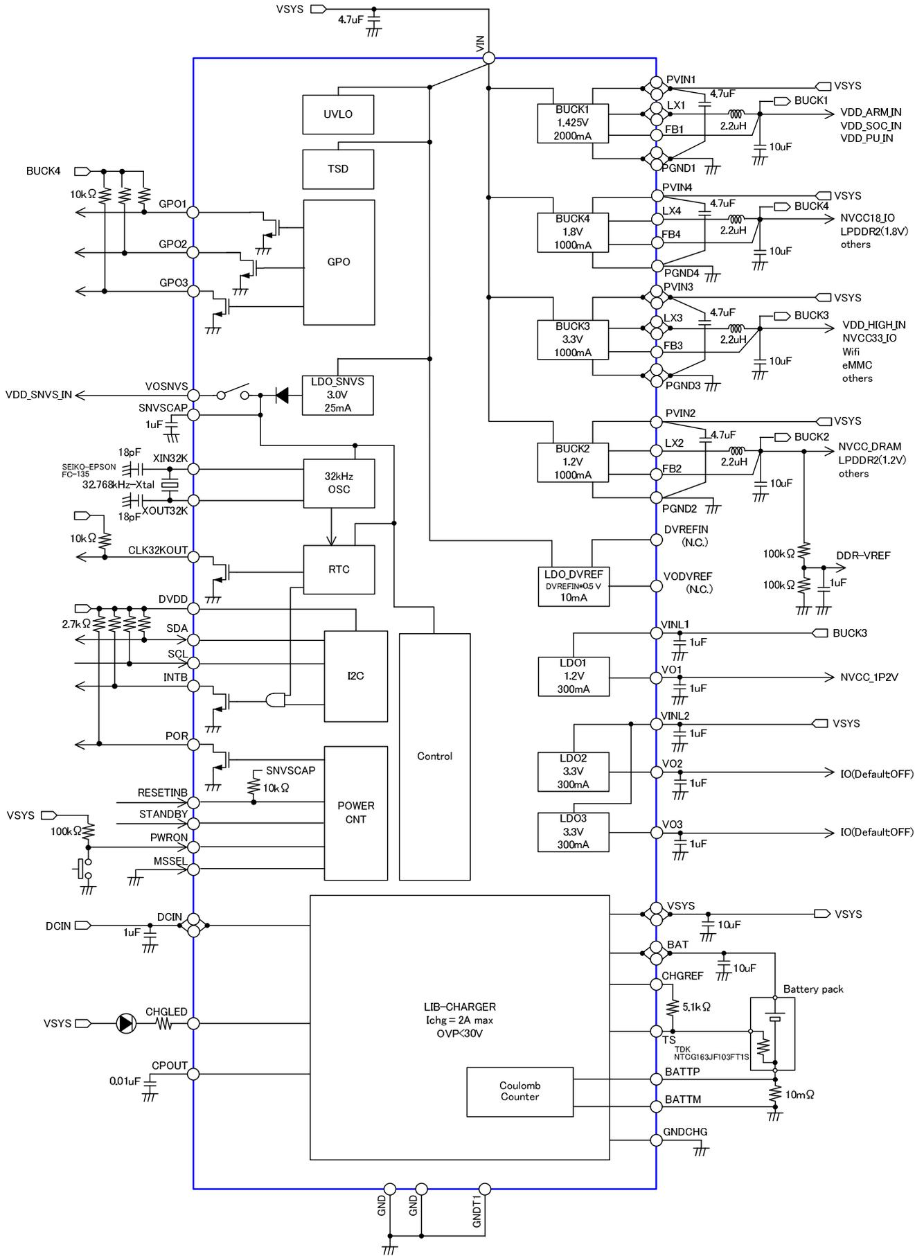
Figure 3. IC Block Diagram (Master Control Mode)
