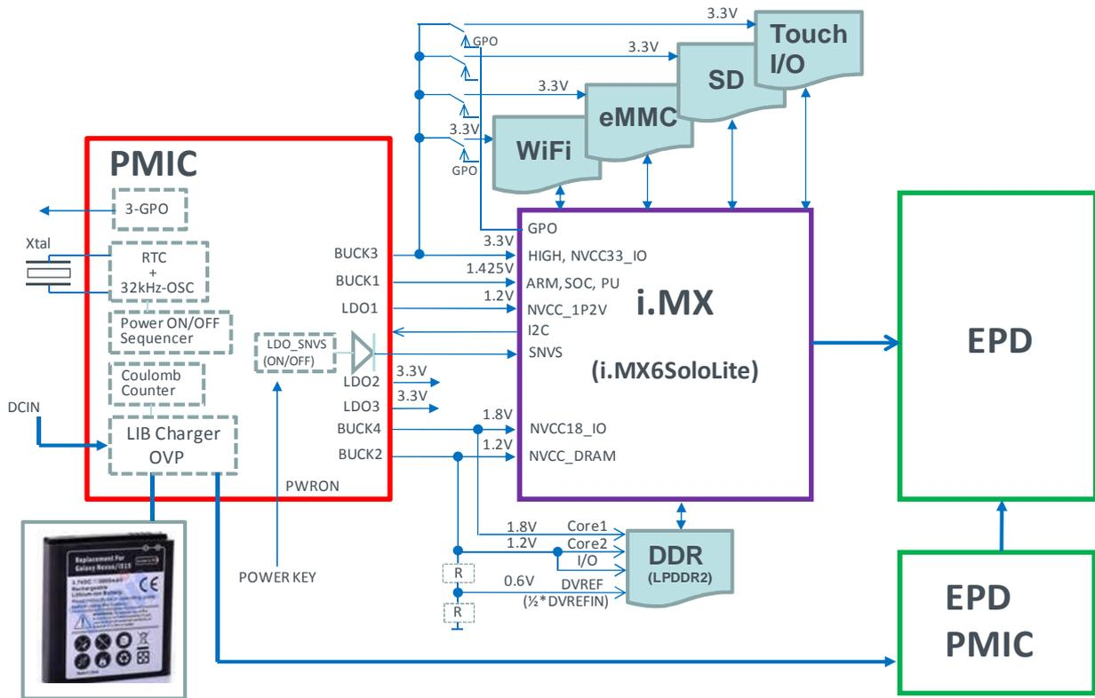
Figure 1. Typical Applications 1 (Master Control Mode)
