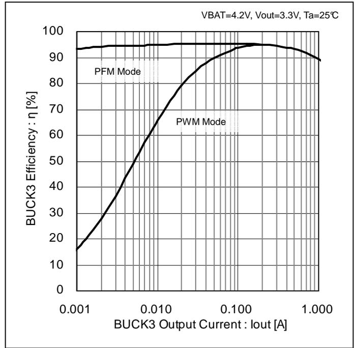
Figure 11. BUCK3 – Efficiency (PWM Mode / PFM Mode)
