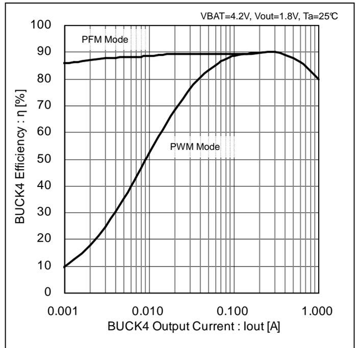
Figure 13. BUCK4 – Efficiency (PWM Mode / PFM Mode)
