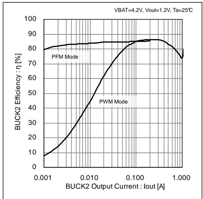
Figure 9. BUCK2 – Efficiency (PWM Mode / PFM Mode)
