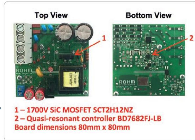
Fig. 2: Top and bottom views of the ROHM AUX evaluation board
