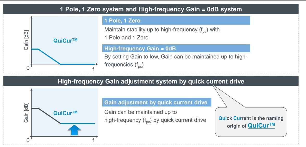
QuiCur<sup>™</sup> is made by the advanced combination of two core technologies
