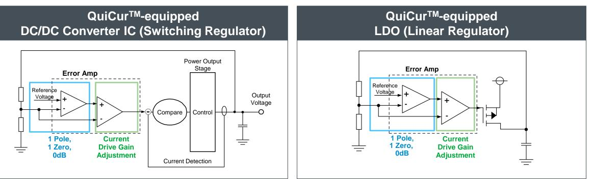
Integrates Two dedicated Error Amps 1<sup>st</sup> Stage Amp: 1 Pole, 1 Zero system and High-frequency Gain 0dB system
