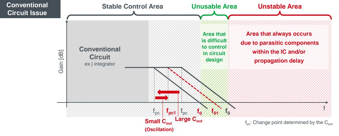
Conventional Circuit has often constrained response performance by Output Capacitance
