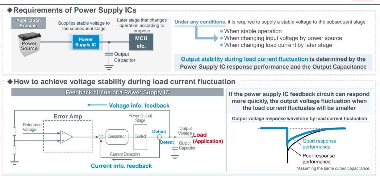
Power Supply IC constantly monitors the output voltage and compares the information with the reference voltage to return the output voltage to the desired value even when the load current fluctuates
