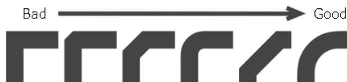
Figure 15. Layout of corner wiring
