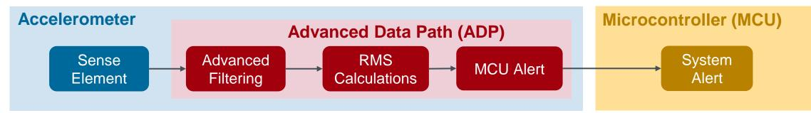
Take Away Message: KX132-1211 & KX134-1211 are designed to perform vibration analysis at a fraction of power compared to a microcontroller to perform a similar task!
