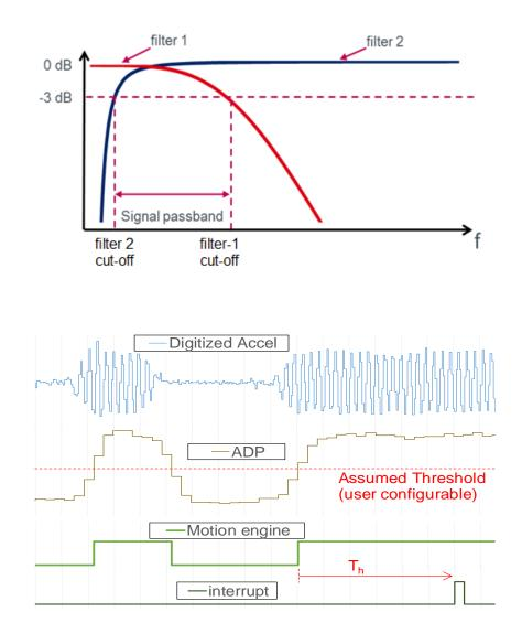
**Step 2 (optional**): To estimate the amplitude of the vibration, the input signal can be routed via a configurable RMS engine where as many as 2 to 256 samples can be averaged. The resulting signal amplitude (and duration) can be used to compare against a configurable threshold to confirm if it exceeds it or not.
