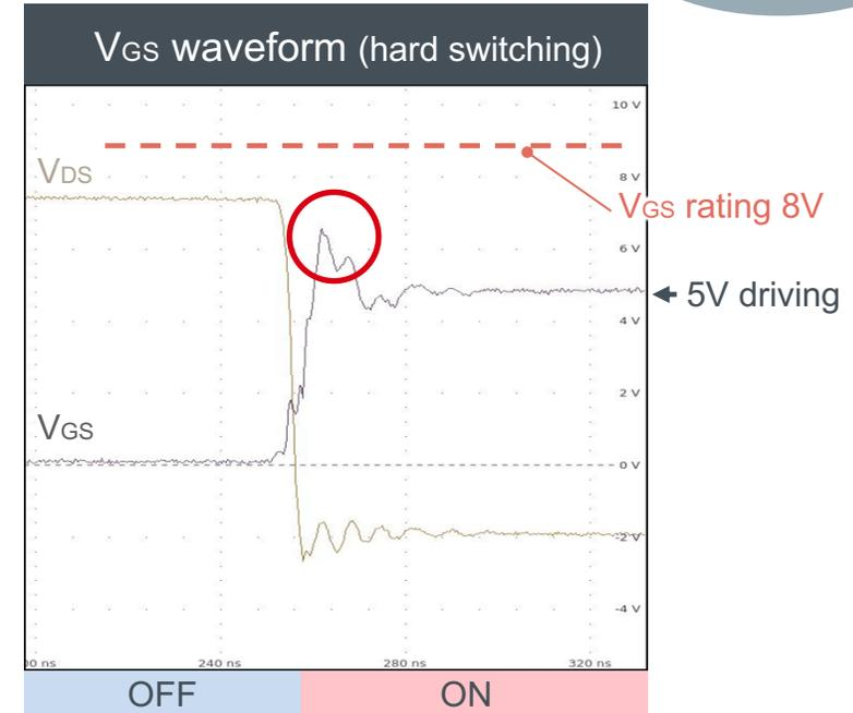
Even if the overshoot voltage occurs, the margin that does not exceed rated voltage is secured to ensure reliability.
