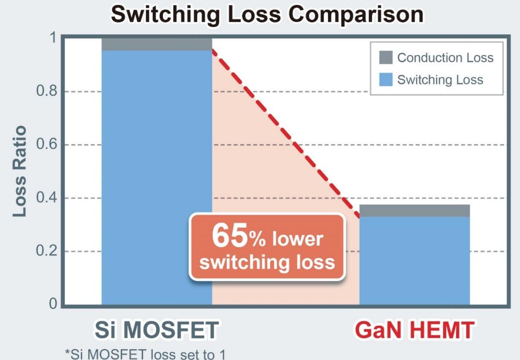
**GaN HEMTs can significantly reduce switching losses compared to Si MOSFETs**
