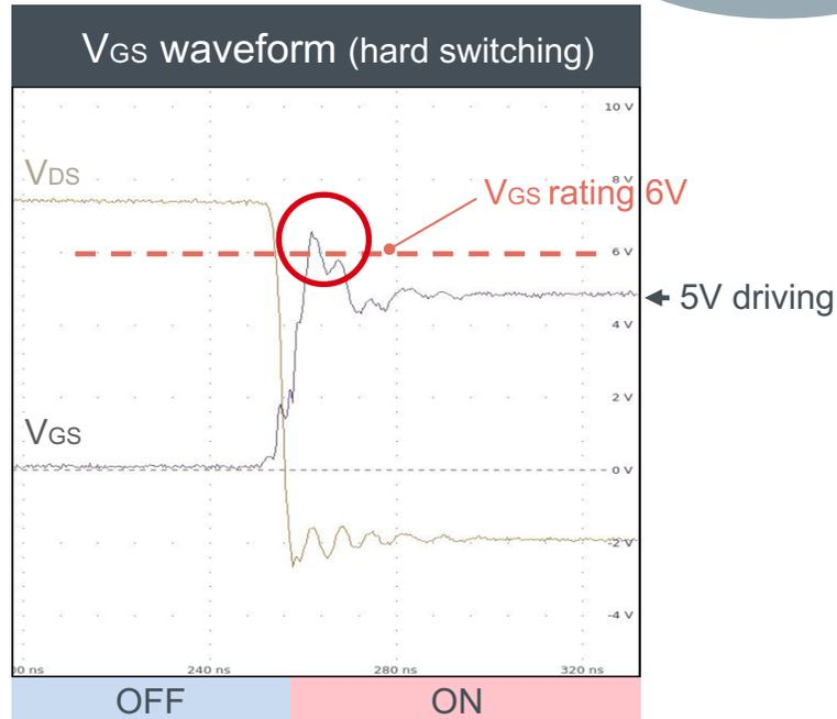
When the overshoot voltage is generated, rated voltage may be exceeded, causing problems with device reliability.
