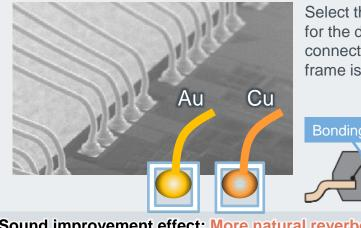
Select the best bonding wires material for the device because its material that connecting the device to the lead frame is affected the sound quality
