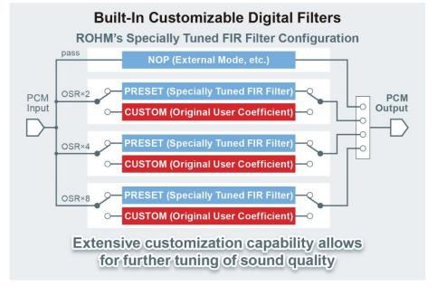
Customizable digital filters help reduce development load and create the ideal sound sought by manufacturers
