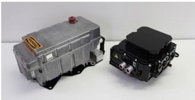
Figure 5: Two power train inverters (Si IGBT based 200kW inverter and SiC MOSFET based 220kW inverter)
