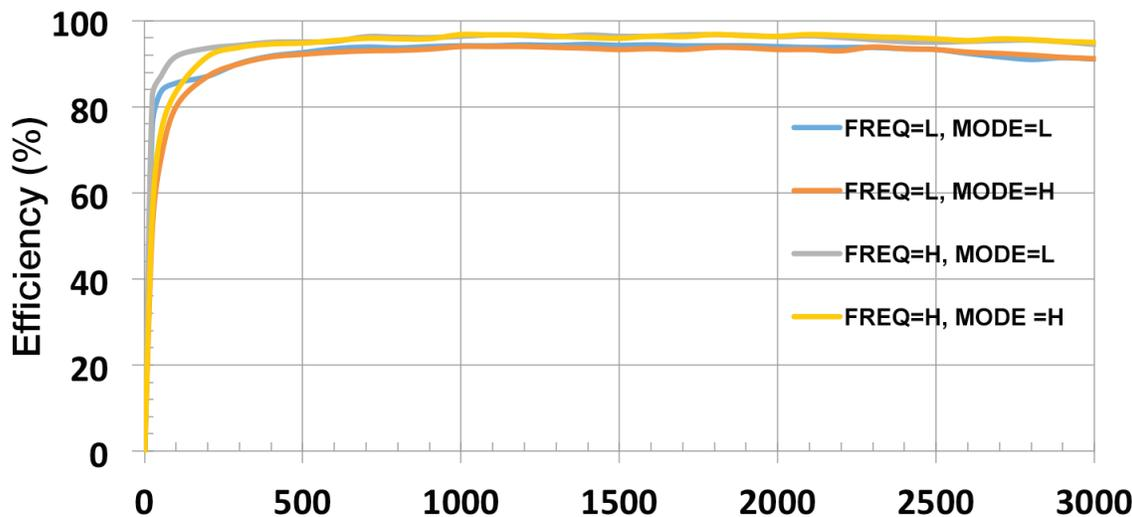
Efficiency Curve for the BD9B300MUV ( $V_{in} = 5V$ ,  $V_{out} = 3.3V$ )
