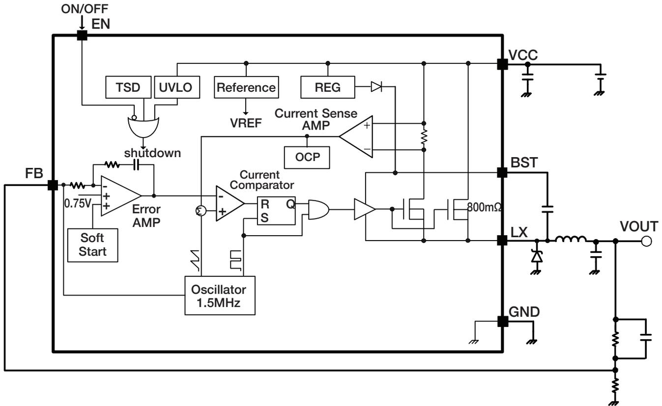
Figure 4: Block Diagram of ROHM's BD9G101G Step-Down Switching Regulator with Built-In Power MOSFETs
