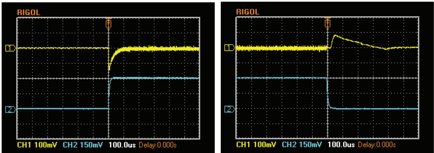
( $V_{in} = 5V$ ,  $V_{out} = 3.3V$ ,  $I_{OUT} = 0A \rightarrow 3A \rightarrow 0A$ , FREQ=L, MODE=L).
