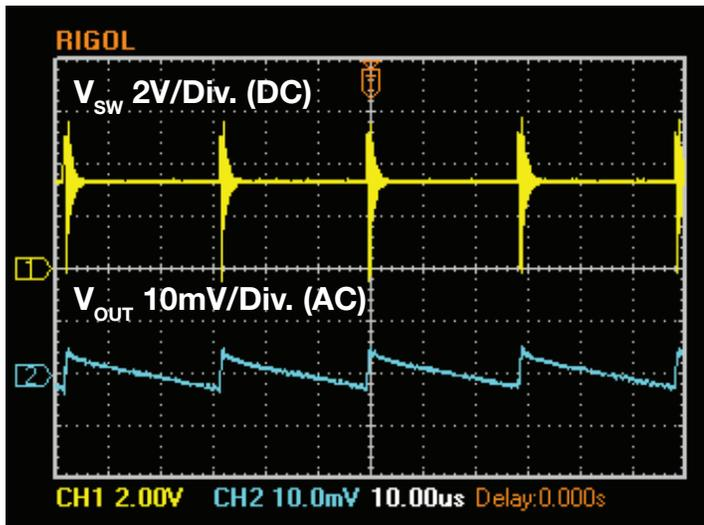
$V_{in} = 5V$ ,  $V_{out} = 3.3V$ ,  $I_{out} = 0A$ , PFM Mode
