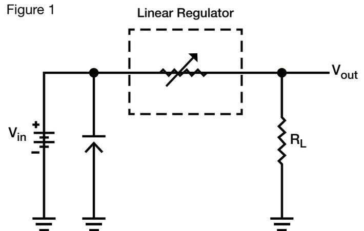
As shown in Figure 1, a linear regulator is nothing more than a variable resistor whose resistance varies based on the output load resistance in order to provide a constant voltage.
