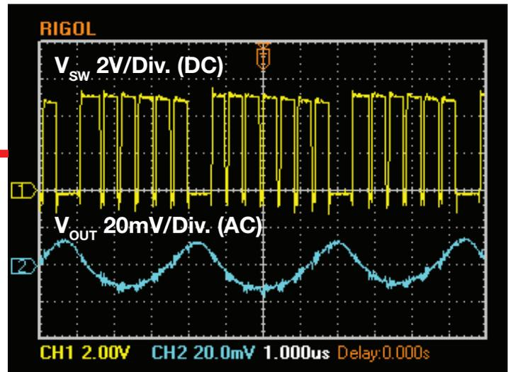
$V_{in} = 5V$ ,  $V_{out} = 3.3V$ ,  $I_{out} = 3A$ , PWM Mode
