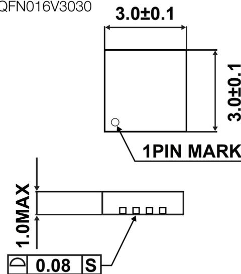
Figure 6: Examples of Small Packages Offered in ROHM's DCDC Switching Regulator Lineup
