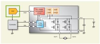
Figure 7. With a DAC, a digital voltage converted to analog can provide the  $V_{_{REF}}$  input.
