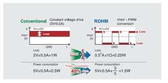
Figure 2. Comparison of linear vs. PWM implementation. In the linear implementation, at anything but full speed, the voltage drop across the control transistors results in significant power dissipation.
