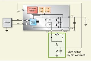
Figure 8. Adding a soft-start function simply requires adding a capacitor and two diodes.
