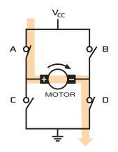
Figure 1. Simplified H-bridge Schematic
