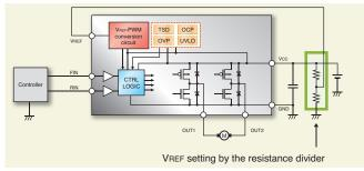
Figure 5. Simple analog speed control using a voltage divider input.
