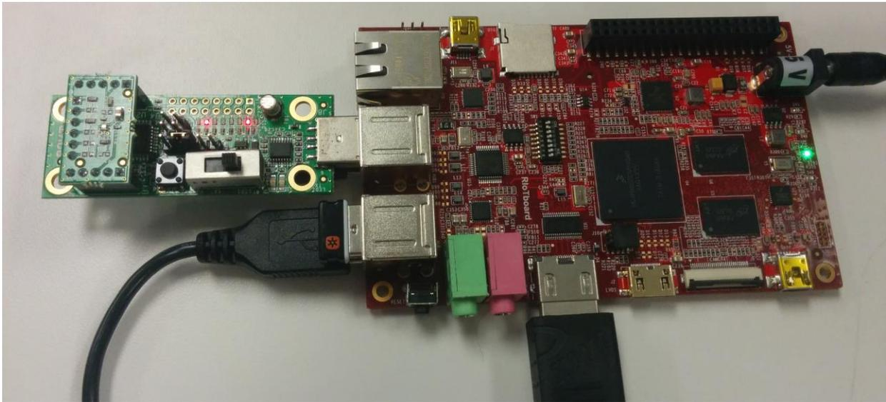
Above: ROHM Sensor Platform Base Board connected to the RioTboard
