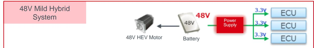
**Power supply ICs are required to output a low output voltage from a high input voltage**
