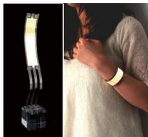
Flexible organic EL devices feature significantly reduced thickness and weight compared to conventional products, enabling the development of new products, such as personal lighting accessories.
