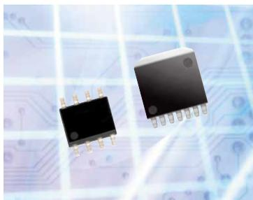
ROHM integrated a switching regulator circuit and a power MOS FET into a single chip to develop ICs that can be used as easily as 3-terminal regulator ICs. The newly developed switching regulator ICs have a remarkably high conversion efficiency of 90% or more. ROHM offers an extended lineup of these ICs with a wide input voltage range of up to 50 V, enabling customers to incorporate them into products requiring high input voltage, such as plasma TVs and office automation equipment.
