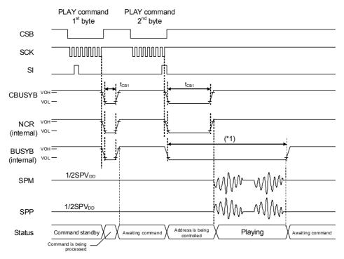
Note: The time length of "L" level of BUSYB is  $t_{\text{CB1}}$  + voice reproduction time.
