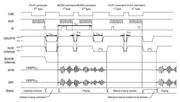
\*1: The time length of "L" level of the NCR signal during playback or silence insertion varies depending on the input timing of command.
