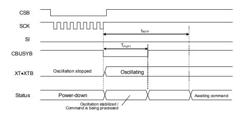
The regulator output starts operating after the PUP command is entered. Any command will be ignored if entered while oscillation is stabilized. However, if a "L" level is input to the RESETB pin, the LSI enters a power down state immediately.
