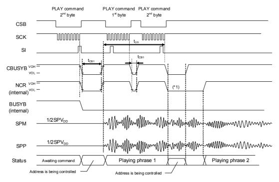
\*1: The time length of "L" level of the NCR signal during playback varies depending on the input timing of command.
