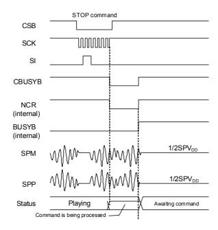
The playback related command (:PLAY, START or MUON), used on after the STOP command, should be input after confirming the completion (: NCR is "H" and BUSYB is "H") of this command processing by the RDSTAT command, or waiting for 12ms from transition of the CBUSYB to "H" level.
