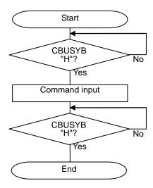
• 2-byte command input flow (Applies to AMODE, AVOL, FADE, FDIRECT, FADR, PLAY, MUON, CVOL, OUTSTAT, SAFE commands.)
