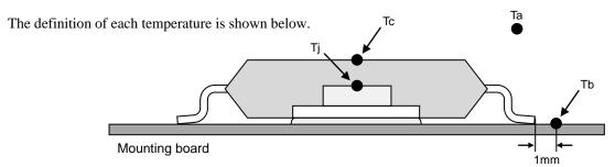
Take measures to dissipate heat on the mounting board so that the maximum junction temperature does not exceed 125 °C.
