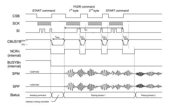
When making continuous playbacks, input the START command for the next phrases within the specified time period (tcm) after the NCR of the corresponding channel changes to "H" level, so that the LSI plays back the next phrases without silence sounds after the current phrase playback ends.
