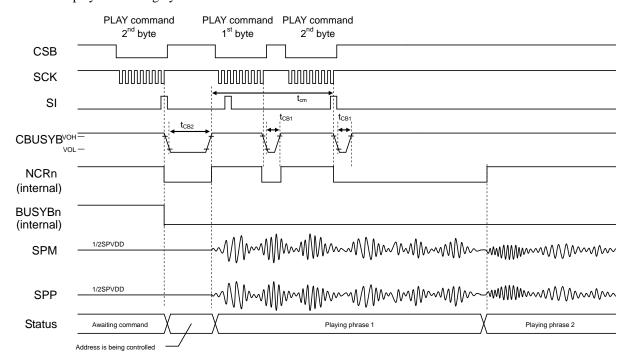
When making continuous playbacks, input the PLAY command for the next phrases within the specified time period (tcm) after the NCR of the corresponding channel changes to "H" level, so that the LSI plays back the next phrases without silence sounds after the current phrase playback ends.
