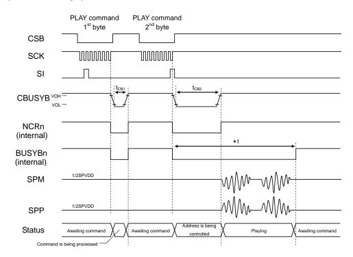
When the first byte of the PLAY command is input, the device waits for the input of the second byte after the command processing time ( $t_{CB1}$ ). When the second byte is entered, the address data of the phrase to be played after the command processing time ( $t_{CB2}$ ) is read from the flash memory.
