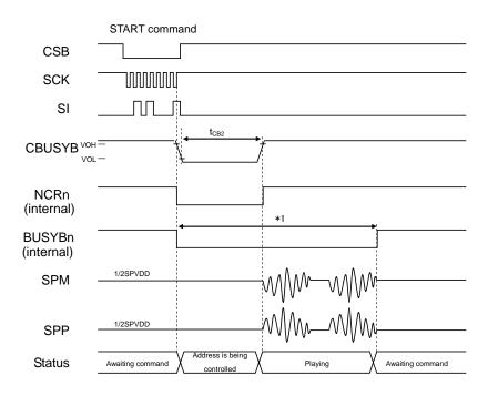
When the START command is input, the address data of the phrase to be played after the command processing time ( $t_{CB2}$ ) is read from the flash memory. When the phrase address data is read, the specified phrase starts playback, and when playback is completed, the BUSYB signal of the playback channel becomes "H" level.
