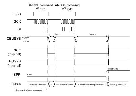
• Speaker amplifier power-down timing (DAMP bit = "0", AEN1 bit = "0", AEN0 bit = "1"  $\rightarrow$  "0")
