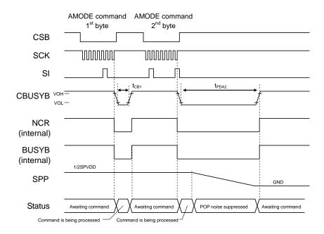
• Line amplifier power-down timing (DAMP bit = "0", POP bit = "0", AEN1 bit = "1"  $\rightarrow$  "0", AEN0 bit = "0")
