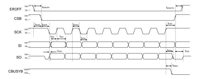
◆ Clock Synchronous Serial Interface Timing (SCK Initial Value = "L" Level)
