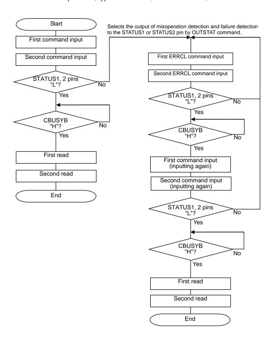
• Read flowchart in two-times input mode (Applies to RDERR command)
