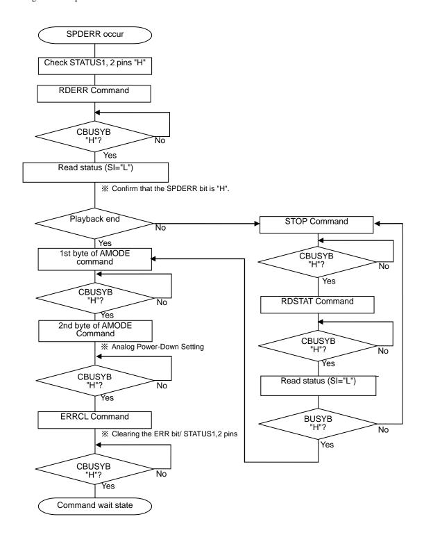
• 1-byte command input flow in two-times input mode
