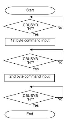
• 3-byte command input flow (Applies to FADR2, PLAY2 command)
