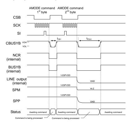
• Speaker amplifier power-down timing (DAMP bit = "1", AEN1 bit = "0", AEN0 bit = "1"  $\rightarrow$  "0")
