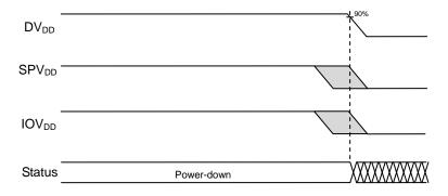
Shut down in order of  $IOV_{DD}$ ,  $SPV_{DD}$ , and  $DV_{DD}$  or  $SPV_{DD}$ ,  $IOV_{DD}$ , and  $DV_{DD}$ . It is possible that the  $IOV_{DD}$  shuts down and then the  $SPV_{DD}$  and  $DV_{DD}$  shut down at the same time, or the  $SPV_{DD}$  shuts down and then the  $IOV_{DD}$  and  $DV_{DD}$  shut down at the same time. The  $DV_{DD}$ ,  $SPV_{DD}$  and  $IOV_{DD}$  can also shut down at the same time.
