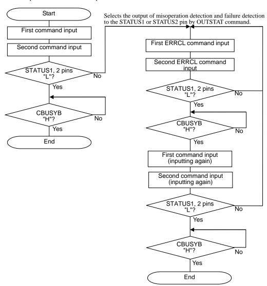
2-byte command input flow in two-times input mode
