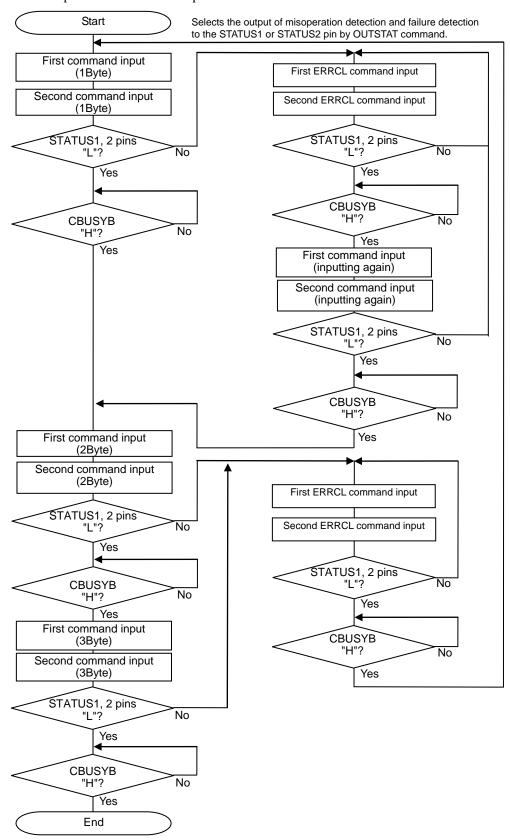
• Read flowchart in two-times input mode (Applies to RDSTAT, RDVER commands)
