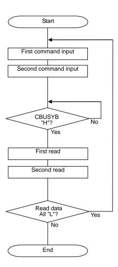
When the OUTSTAT command is used to select the misoperation detection and failure detection outputs and the STATUS1 or STATUS2 pin is "H", if all the read data is "L", the data cannot be read normally. Read the data again.
