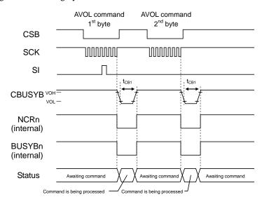
Speaker amplifier volume setting by AVOL commands is valid only when Class AB speaker amplifier is used. When a Class D speaker amplifier is used, the setting value is ignored and +0.0dB is selected.
