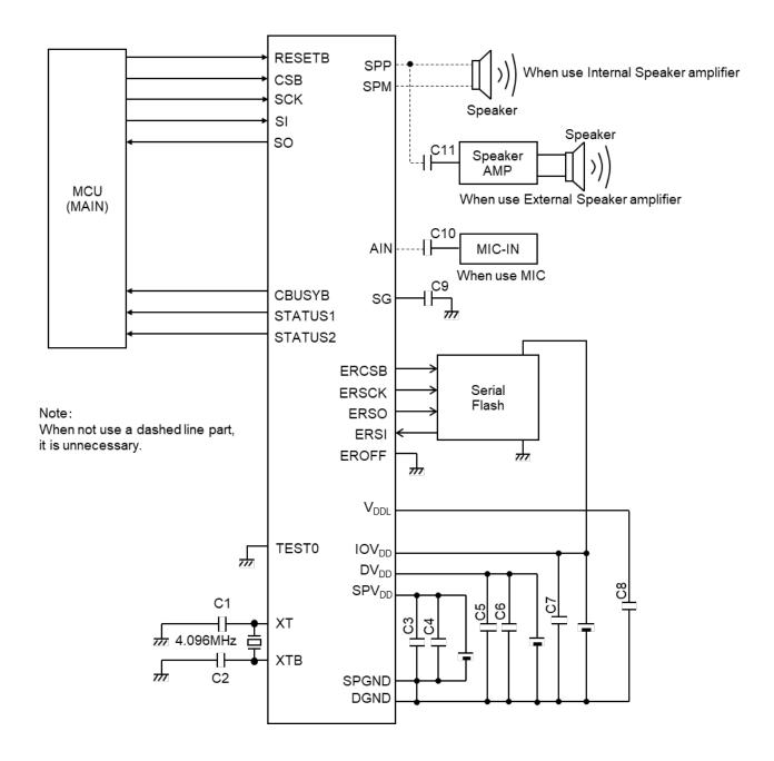
Please add necessary bypass capacitor to a power supply pin of the serial flash memory separately. The power supply for the ERCSB, ERSCK, ERSO, ERSI and EROFF pins is  $IOV_{DD}$ . If the crystal unit has a built-in capacitor, C1 and C2 are not needed.
