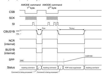
• Line amplifier power-up timing (DAMP bit = "0", POP bit = "0", AEN1 bit = "0" → "1", AEN0 bit = "0")
