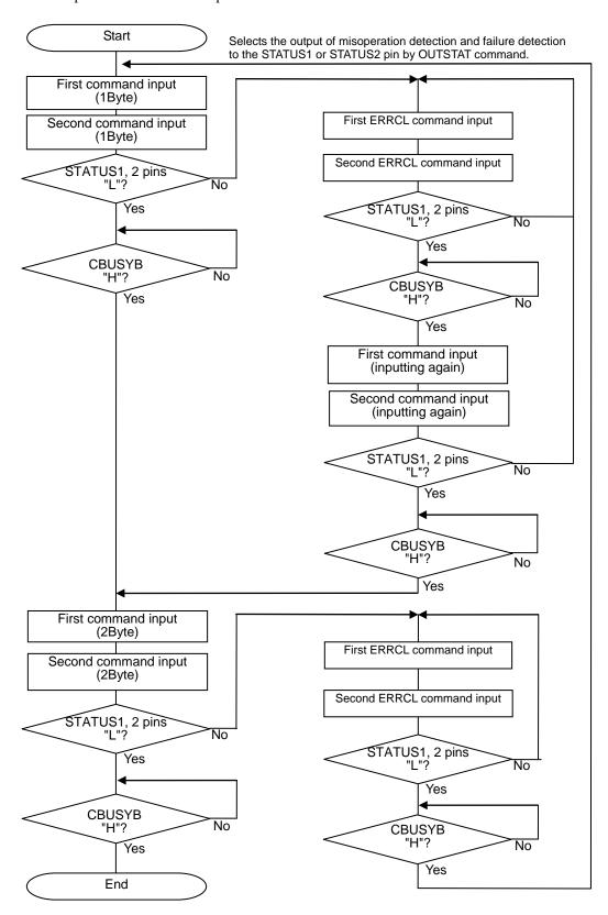
• 3-byte command input flow in two-times input mode
