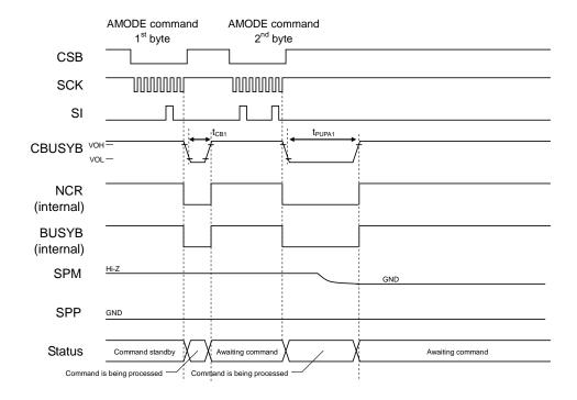
• Line amplifier power-up timing (DAMP bit = "0", POP bit = "1", AEN1 bit = "0"  $\rightarrow$  "1", AEN0 bit = "0")
