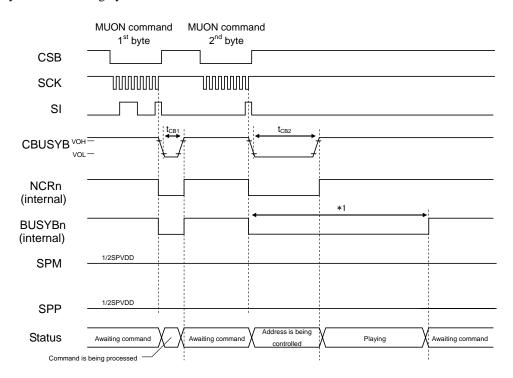
When the first byte of the MUON command is input, the device waits for the input of the second byte after the command processing time ( $t_{CB1}$ ). When the second byte is entered, the silence time is calculated after the command processing time ( $t_{CB2}$ ). When the calculation of the silence duration is completed, the calculated silence is played back, and when the playback is completed, the BUSYB signals of the playback channels become "H" level.
