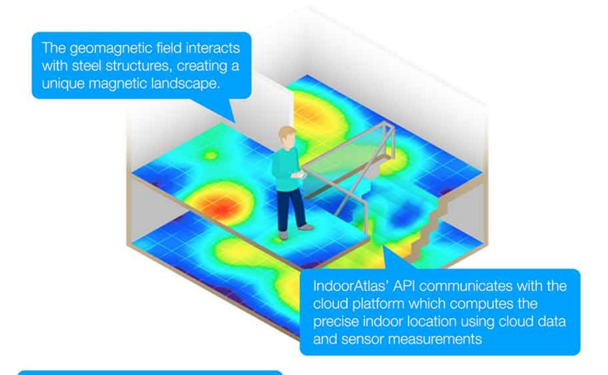
Leveraging sensors built into smartphones allow the magnetic field and radio signal landscapes to be measured and sent to the IA cloud
