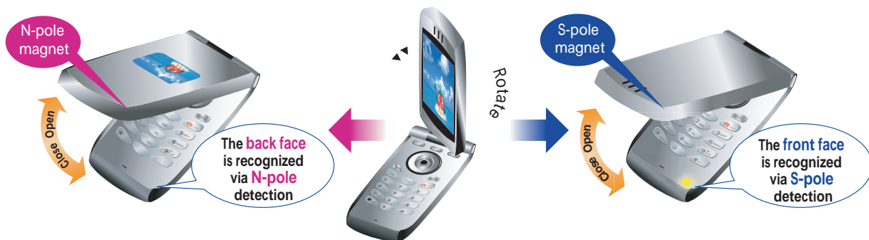
Figure 3. Polarity-discriminating Omnipolar Hall effect IC switches can be used to control the operation and orientation of multiple displays
