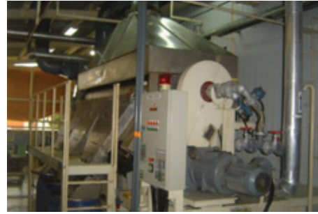
Drum dryer in a closed treatment facility
