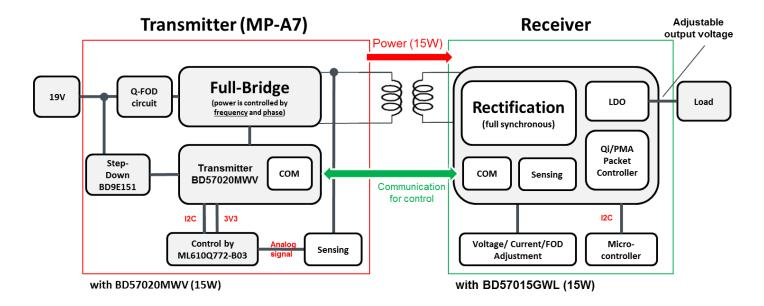
Figure 1: Design Kit Block Diagram
