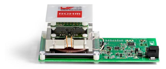
Figure 3: Stacked RX+LED Module placed on coil area of TX Module
