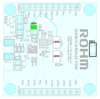
Figure 5: Receiver Module, top view
