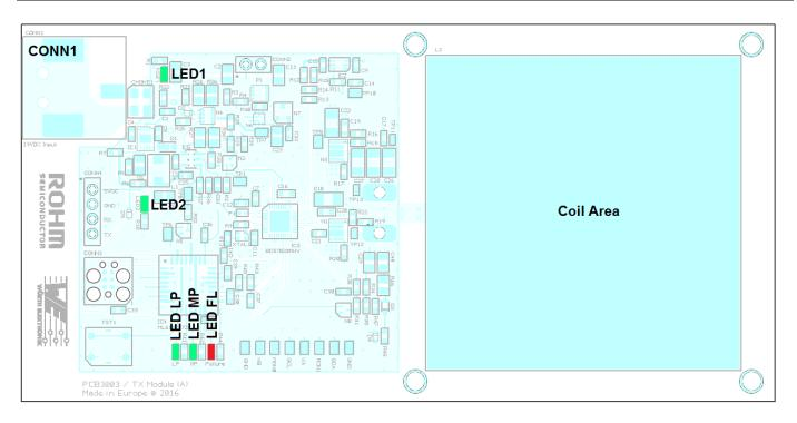
Figure 4: Transmitter Board with indication of inputs, outputs and status LEDs
