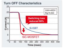
SiC not only provides greater energy savings and efficiency, but also enables smaller peripheral components to be used during high-frequency (30kHz over) operation, contributing to end-product miniaturization.
